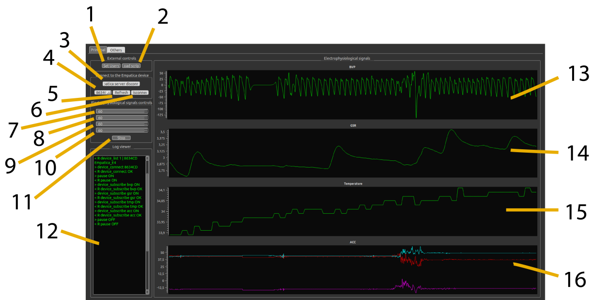
Figure 3.1: BIOSIGNALS: General physiological experimentation in real-time, an open source software for real-time physiological signals acquisition and processing with the Empatica E4 wristband.
