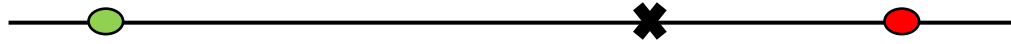
Figure 5.2: Here the green circle would represent non-disruptive centroid c_1 and the red circle would represent disruptive centroid d_1 with X being the point defined by x_1 in equation 3. In a nutshell, if a plasma state point has co-ordinate value higher than the average of disruptive and non-disruptive centroid value, the plasma will be characterized to be in a disruptive state and non-disruptive otherwise and hence, a threshold value.
