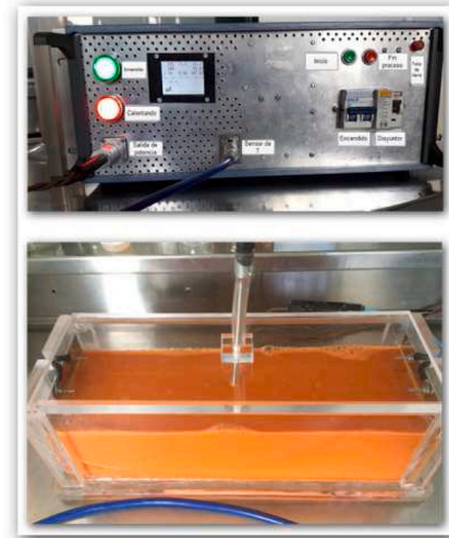
Fig. 1. Block diagram of the ohmic heater and picture of the ohmic heating cell, temperature sensor and voltage signal generator.
