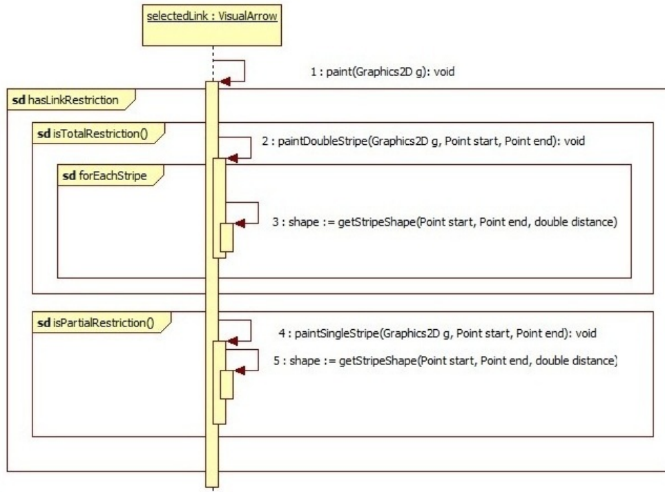
Figure 4.6: Diagram for the painting of a link restriction.
