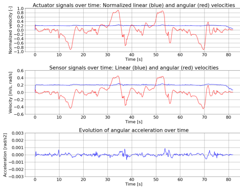
Figure 5.24: Angular speed, angular acceleration, and linear speed. Circuit without obstacles, safety + legal + comfort + task-oriented req. The angular speed, angular acceleration and linear speed correspond to the path of Figure 5.23
