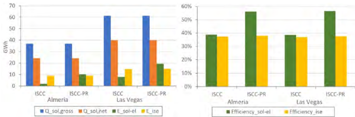
Fig. 8. Solar-to-energy energy conversion (left) and efficiencies (right) for the three configurations in Almeria and Las Vegas.
