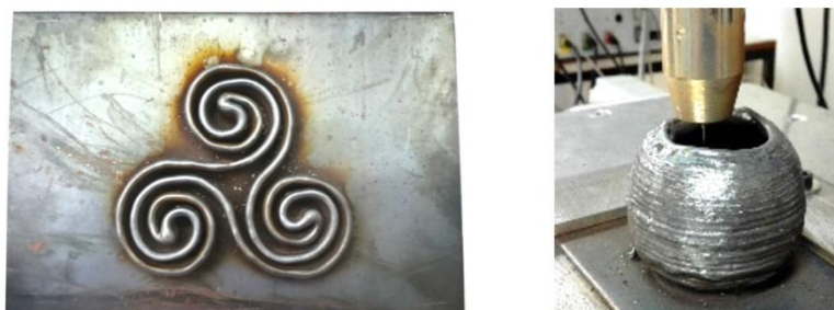
123 124 Figure 2. Examples of geometries obtained by WAAM.
