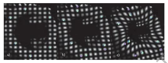
**Fig. 3.** (a) First frame (b) fourth frame and (c) eighth frame of the sequence of the simulated data. Blue triangles are manually tracked points, magenta circles are the points obtained with the HARP method and the green diamonds are the points obtained by the variational method enhanced (For interpretation of the references to color in this figure legend, the reader is referred to the web version of the article).
