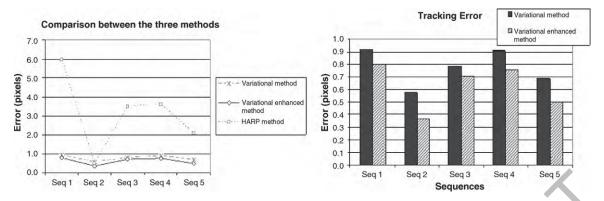
Fig. 5. (a) Comparison of the average tracking RMS error for the five sequences tested when the different methods, variational (asterisk), enhanced variational (diamond), and HARP (square) are used. (b) Average tracking RMS error for the five sequences tested with the variational (flat color) and enhanced variational (grated) method.
