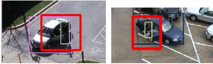
Figure 27: Examples of ground truth from VIRAT database where both the person and vehicle bounding boxes are plot in different colours, and the event boxes are marked by thick red box.
