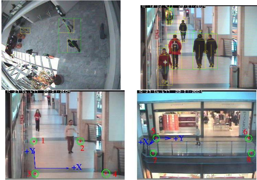
Figure 5: Examples of typical frames in CAVIAR dataset: frame recorded at INRIA Labs (left top), example of a marked up frame with identification heads, gaze, hands, feet and shoulders recorded at the hallway in a shopping center in Lisbon (right top) and examples of two frames synchronized along (left bottom) and across (left right) the same corridor, showing ground plane homography data.
